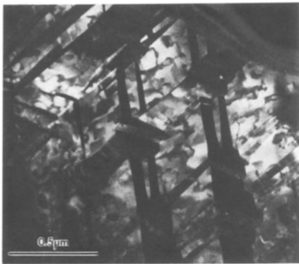
Figure 5 Double-exposed print of the micrographs in Figs 4b and c. Two variants of t' -ZrO 2 are brightly imaged. The domain structure is not continuous in two adjacent variants.
